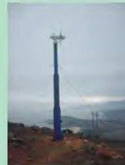
This project use our electronic yawing type 4pcs of 5kw wind turbine systems, this kind of wind turbine without tail but with wind vane, anemoscope ... Until now, it works well and be popular among local residents.
